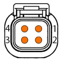
Pins 1 and 4 for supply (thicker traces), current limit 7,5A
