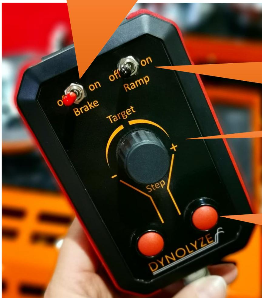
When you switch on "Ramp" (brake needs to be on) it will start your selected brake program (sweeping up, Drive Simulation etc..). You can set a desired ramp in the Brake Control settings under the menu: "RPM and Brake settings F5"
